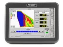
**Field computers** allow farmers to control the application of fertilizers, herbicides, and pesticides through automated delivery systems.
